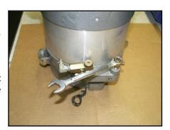
Use ¼" NPT Plug Fitting (preferably Brass) to plug the vent valve port. Apply Teflon tape or an equivalent sealant (ex. Staybond S592) to the fittings threads. Then tighten the plug fitting into the vent valve port.
