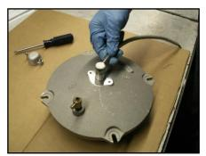
After the heating element has been removed, place the heater cover back on the TF Lid. Position screws in place and tighten heater cover screws down with 12 in-lbs. A small amount of Loctite can be applied to prevent the screws from vibrating loose in the future.
