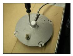
Using a Philips screwdriver, unscrew the two heater cover screws. Remove Heater Cover from the TF Lid, being careful not to lose the 2 screws as they will be needed later to reinstall the heater cover.
