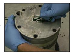
With one hand grab and "push" the wire through the channel. This may require a screwdriver to leverage the wires up before pulling wires by hand. Be careful not to scar the wire insulators.
