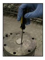
To remove the heating element, it is best to remove the puraDYN system from its mounting location to access the bottom of the PFT Unit where the heating element is located.
