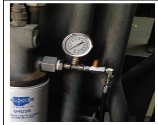
Picture 6 (Oil supply Shut-valve- MTU16V2000) (Pressure gauge setup not part of kit)
