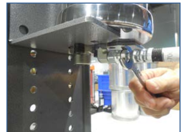
8) Reconnect hose assembly, and check all fittings for tightness
