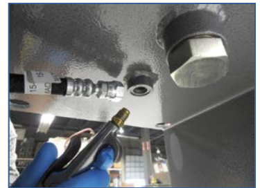
4) Clean port internals & metering jet screen with solvent/fine wire brush; use high-pressure air to blow-out port & screen, clearing any debris
