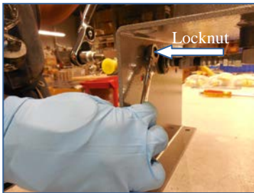
1) Loosen locknut, which secures FPS Manifold Assembly to unit base
