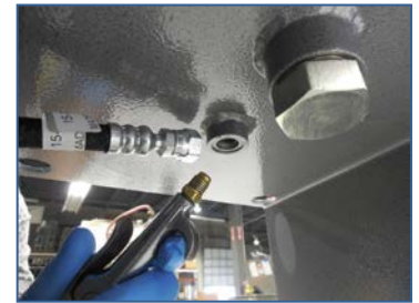
4) Clean port internals & metering jet screen with solvent/fine wire brush; use high-pressure air to blow-out port & screen, clearing any debris
