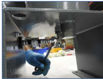
2) Loosen hose fitting, to disconnect 'Inlet Plumbing Hose Assembly'
